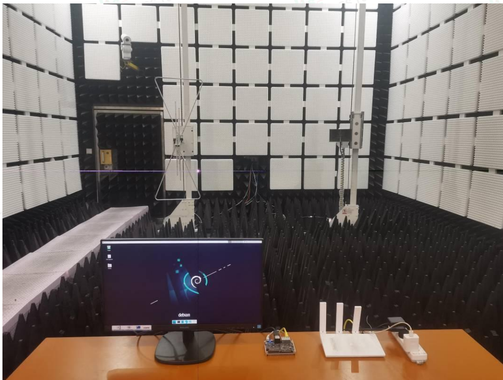
Photo of Radiated emission Measurement(Above 1GHz)
