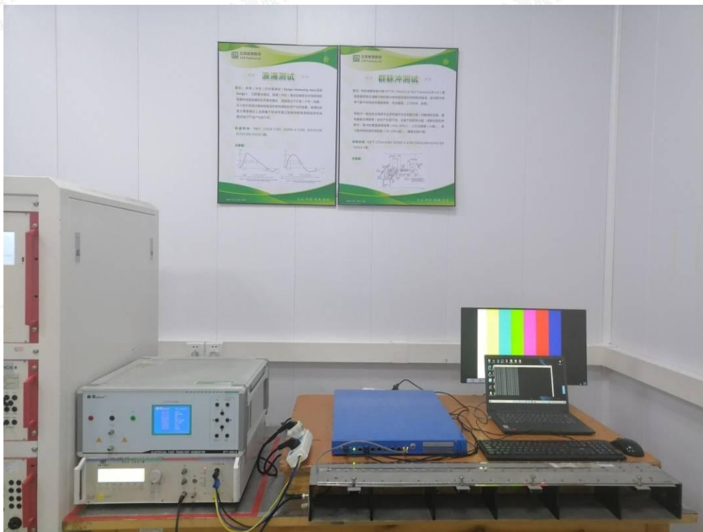
Photo of Signal port Electrical Fast Transient Test Immunity Test
