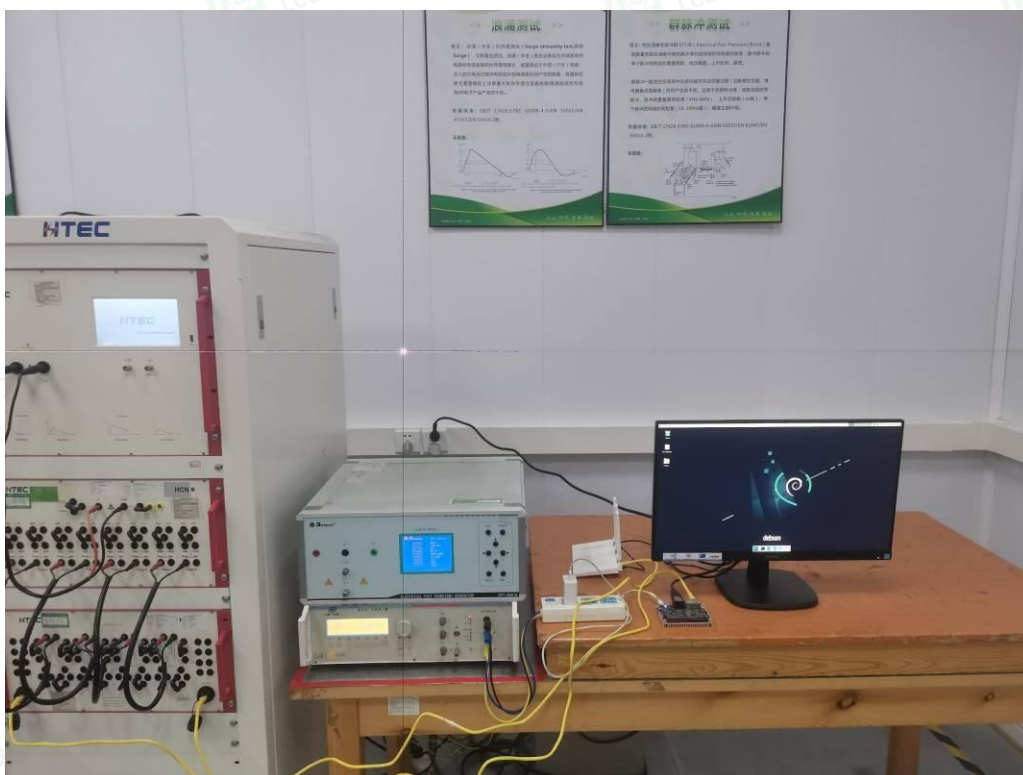
Photo of Signal port Burst Surge Test Immunity Test
