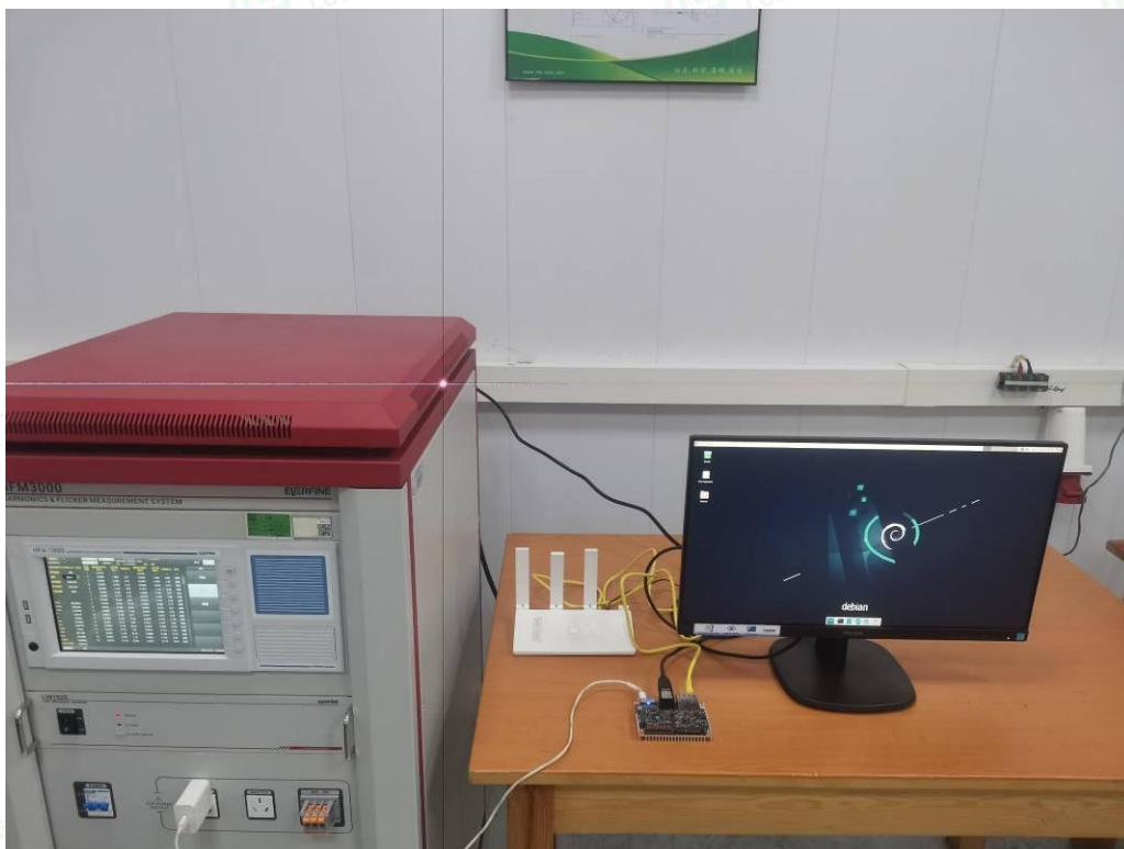
Test Setup Photo of Harmonic & Flicker Measurement
