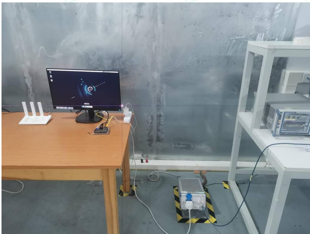
Photo of Power Line Conducted Measurement
